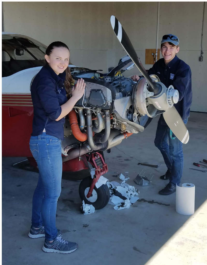
Annie and Liam working to remove a prop governor on a customer's aircraft.
