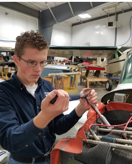
Zack reinstalling and torquing spark plugs during an Annual Inspection on a customer aircraft.
